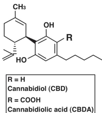
**Fig. 1.** Chemical structures of CBD and CBDA. The chemical structures of CBD and CBDA are shown. CBD (R = H) is formed from CBDA (R = COOH) by decarboxylation (–COOH).
